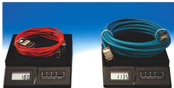
A 100-m fiber-optic cable weighs only 180 g, considerably less than its copper counterpart (1135 g). Courtesy of Intel.
